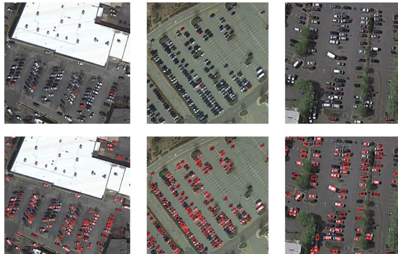
Fig. 1: Vehicle Detection Using YOLO v5
