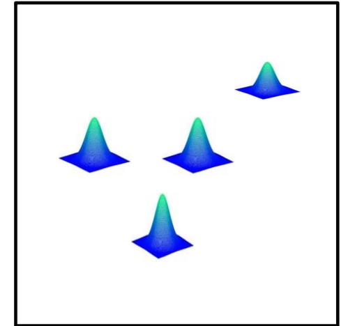
The interaction of a DD domain pulse with a doubly spread channel is predictable, as long as the delay domain period  $\tau_p$  is greater than the channel path delay spread, and the Doppler domain period  $\nu_p$  is greater than the path Doppler spread:
