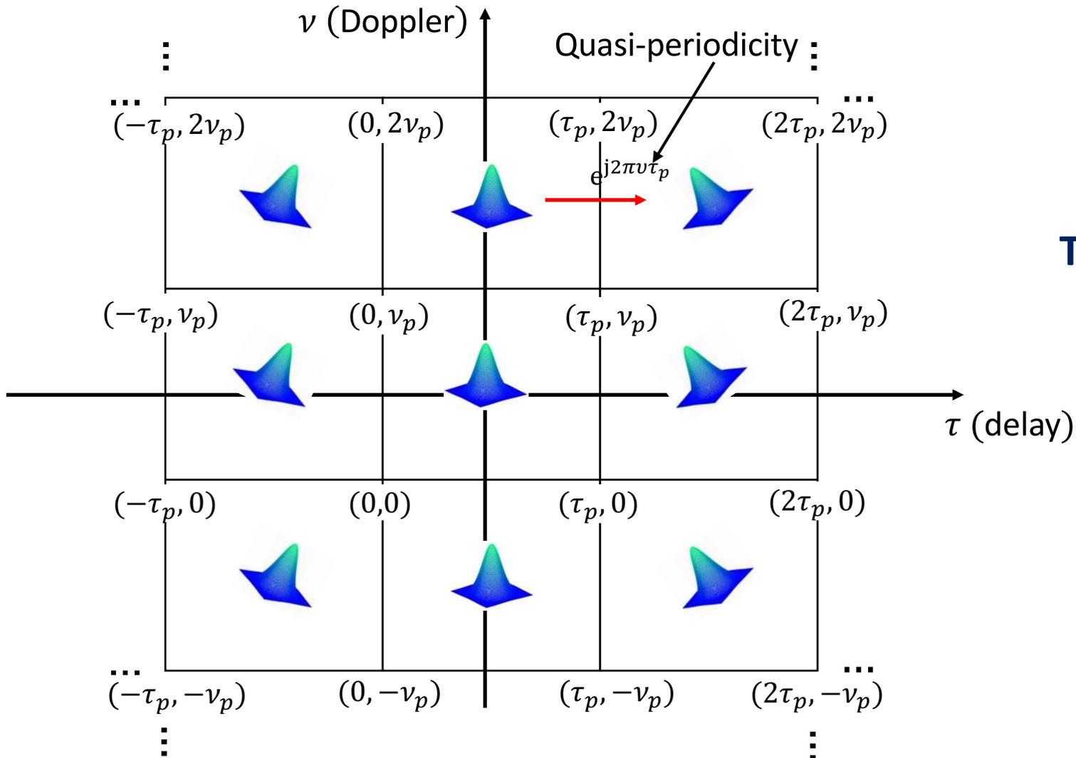
**The DD realization of a TD signal is a quasi-periodic function**
