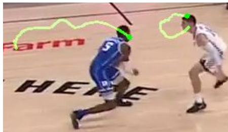
Output of OpenCV Optical Flow algorithm
