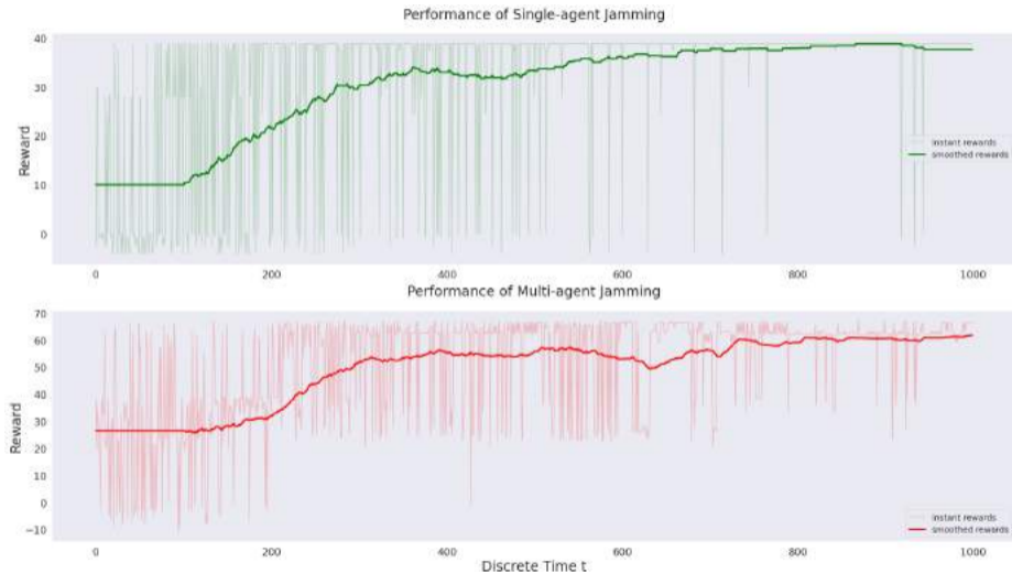
Figure 6: Performance of Jamming vs. Discrete Time Under Sweep Changes of Multi-Channel.
