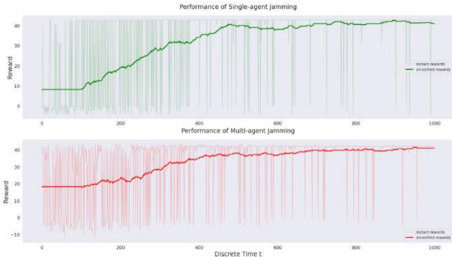
Figure 4: Performance of Jamming vs. Discrete Time Under Sweep Changes of a Single Channel.
