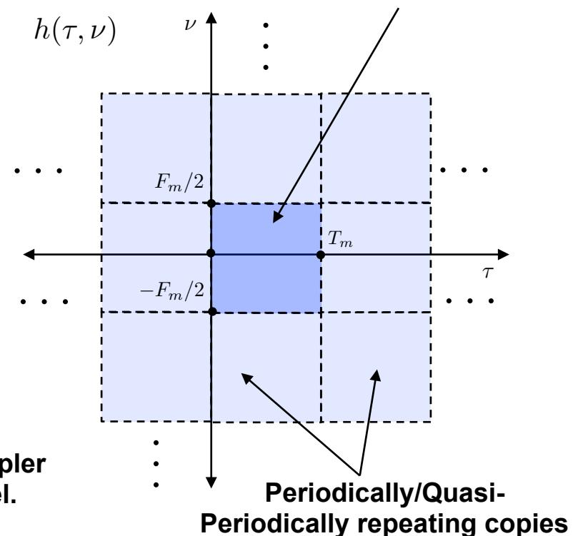
We can interpret the spread function  $h(\tau, \nu)$  as the delay-Doppler response (or Zak response) of the underspread LTV channel.
