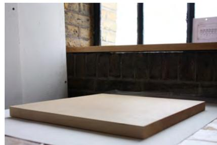
2. Meticulous preparation of the support is essential for a panel on which water gilding will be applied. This starts by covering the panels with layers of glue, which isolate the later layers from the underlying wood, and help in attaching the priming layers. For this reconstruction three layers were applied of different concentrations of rabbit skin glue, heated au bain marie.
