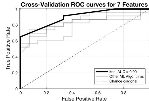
Figure 5: Cross-Validation ROC curves for 5 different ML algorithms (4 features selected to optimize %accuracy)
