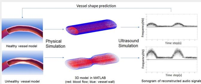
Figure 6: Ultrasound audio signal simulation process
