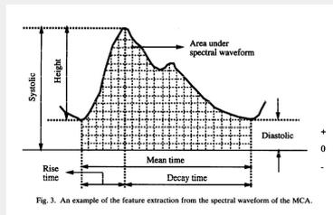
Fig. 3. An example of the feature extraction from the spectral waveform of the MCA.
