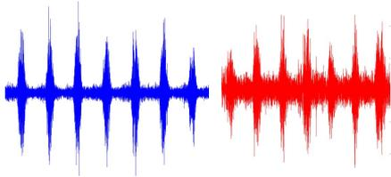
Figure 2: Sample audio signals from ultrasound machine. (a) **Healthy** signal and (b) **Unhealthy** signal
