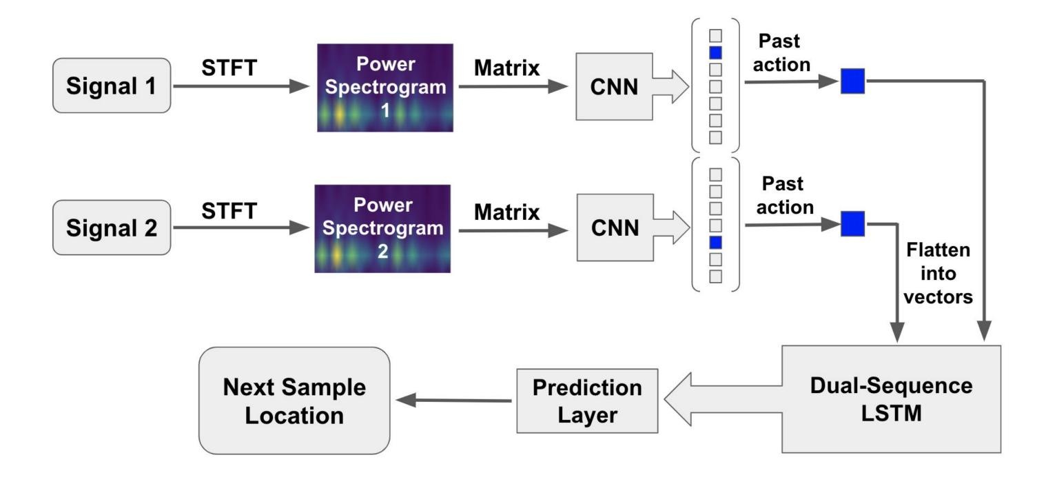
Leverages power spectrograms and a dual-sequence LSTM to predict sample locations.
