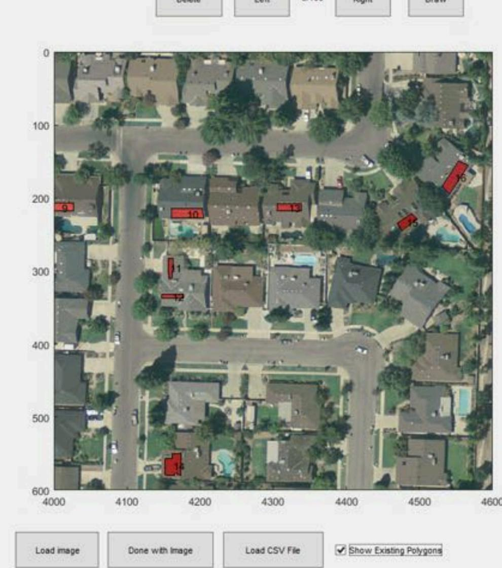
Figure 2: Snapshot of GUI developed for ground-truthing location of solar arrays
