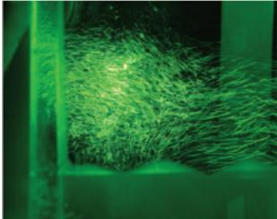
**Fluid Streamlines** (Polystyrene spheres 25  $\mu\text{m}$  in diameter are used as tracers in experiments and illuminated by a laser with)
