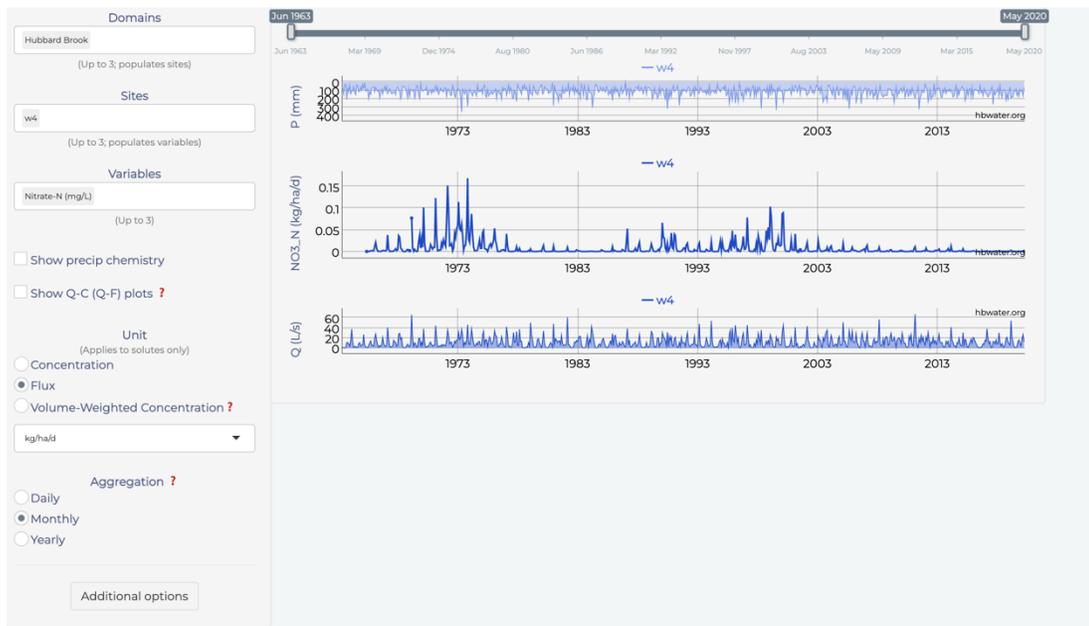
Figure 3: screenshot of dashboard interface, here showing a visualization of long-term nitrate concentrations in water leaving a small watershed. This final lesson used skills
